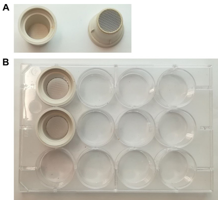
Figure 2. The image of Corning Netwell “immunobasket”. A. The image of immunobasket's top and bottom side. B. The image of immunobaskets mounted on Falcon multiwell plate.
