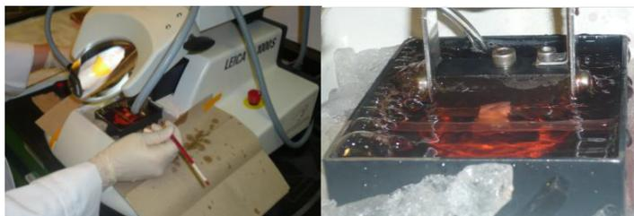
**Figure 1. Use Vibratome to do brain slices**
