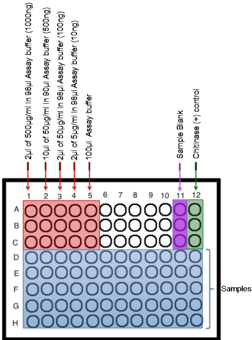
**Figure 1. Plate set-up for chitinase assay.** Red wells indicate 4-Methylumbelliferone standards, Purple indicates the sample blank (Working Solution), Green represents the positive control, and blue wells indicate sample wells.
