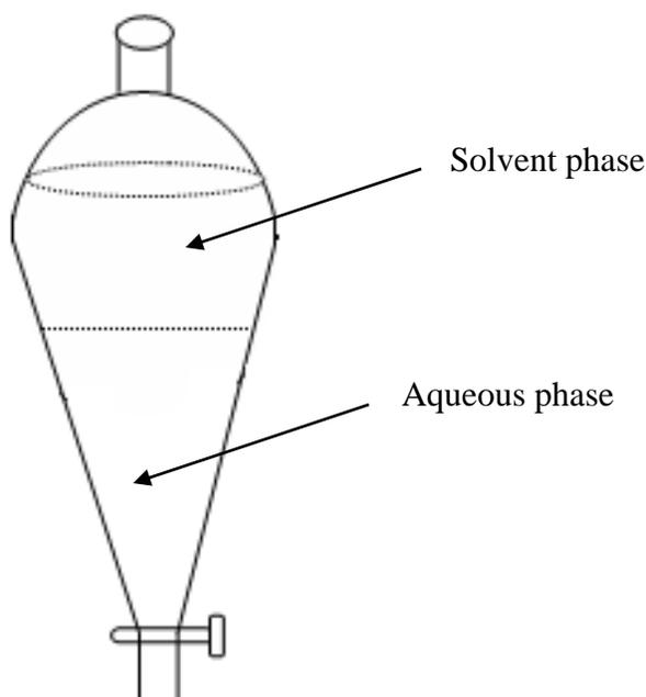
**Figure 1. Partitioning by separator funnel**
