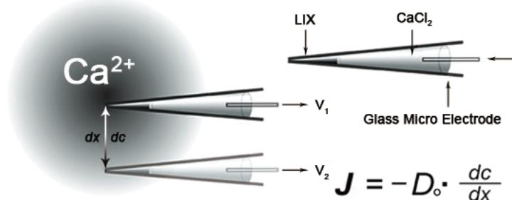
**Figure 1. Schematic diagram of ion flux detection ([www.xuyue.net](http://www.xuyue.net)). The microelectrode tip is filled with liquid ion exchanger (LIX). A voltage gradient ( $dV$ ) is measured by the electrometer between two positions over the travel range  $dx$ . A concentration gradient ( $dc$ ) is calculated based on  $dV$ .  $D_o$ , ion diffusion constant;  $J$ , net ion flux.**
