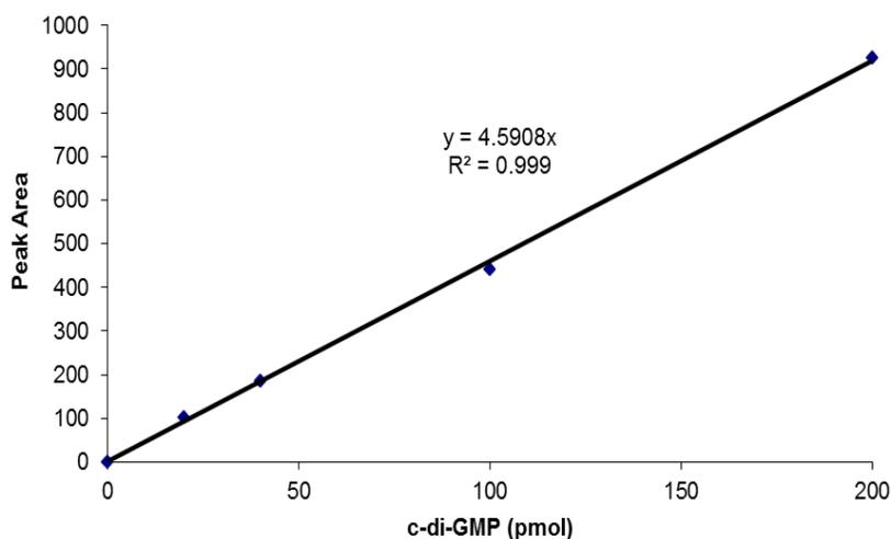
**Figure 2. Example of a c-di-GMP HPLC standard curve.** The standard curve was generated by plotting the peak areas obtained following the separation of 20  $\mu$ l aliquots of c-di-GMP standards (here: 0, 1, 2, 5, and 10 pmol/ $\mu$ l) versus the total c-di-GMP amounts in pmol. Peak areas were obtained using the ChemStation for LC software.
