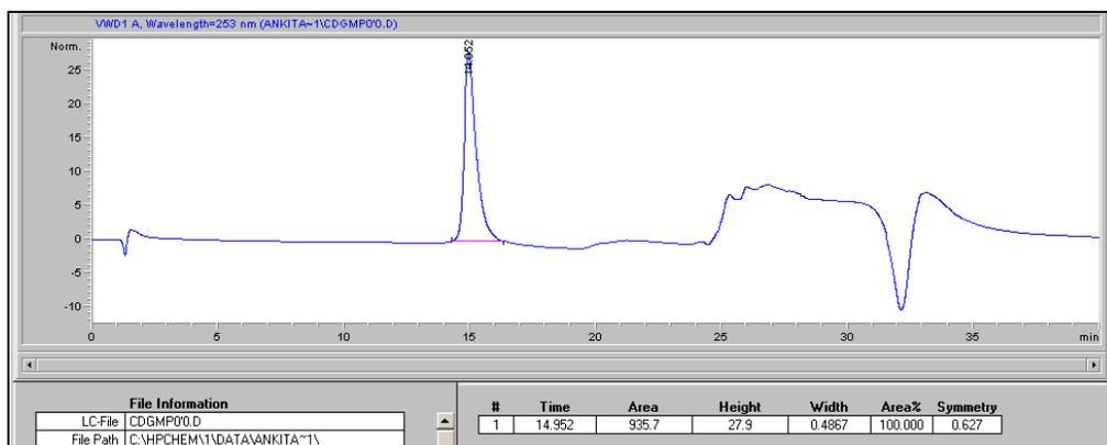
**Figure 1. Example of c-di-GMP standard elution profile.** 20  $\mu$ l of a 10 pmol/ $\mu$ l c-di-GMP standard (200 pmol total) were separated using a reverse-phase C<sub>18</sub> Targa column (2.1 x 40 mm; 5  $\mu$ m) at a flow rate of 0.2 ml/min with the following gradient: 0 to 9 min, 1% B; 9 to 14 min, 15% B; 14 to 19 min, 25% B; 19 to 26 min, 90% B; 26 to 40 min, 1% B. Peak at 15 min corresponds to the elution of c-di-GMP. The c-di-GMP peak was found to have an area of 935.7.
