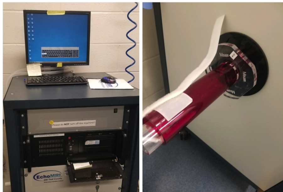
Figure 10. Body composition analysis using EchoMRI
