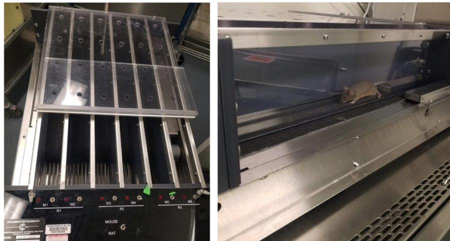
Figure 2. In vivo evaluation of mouse muscle endurance and fatigue by treadmill
