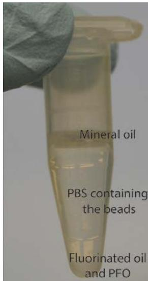
**Figure 3. Three phases after breaking the emulsion**
