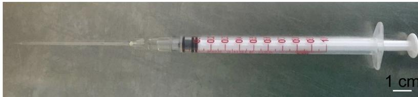
**Figure 1. Glass pipette and syringe coupled together**
