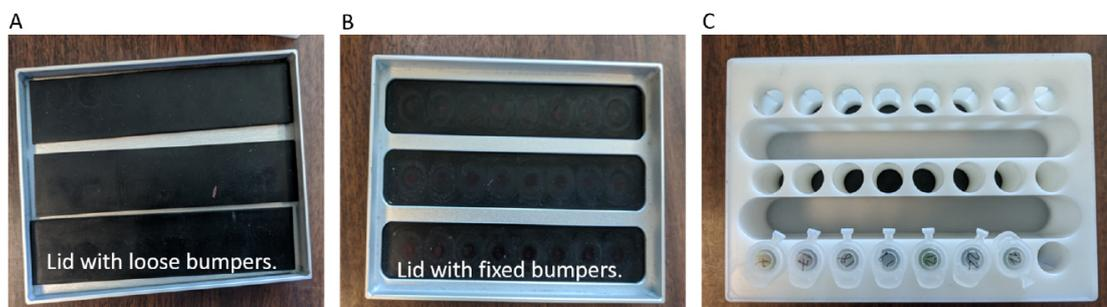
**Figure 2. Parts of the QIAGEN adapter.** A. The lid with loose bumpers; B. The lid with fixed bumpers; C. Tubes loaded into the center, rack portion of the adapter. Note that lids are not overlapping.
