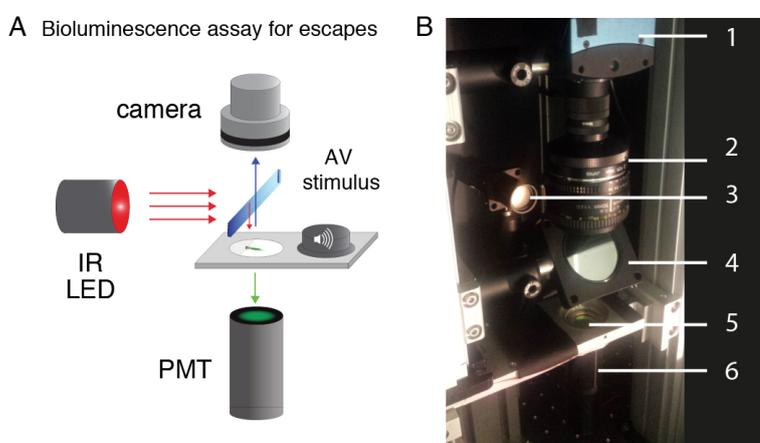
**Figure 2. Bioluminescence setup for escapes.** A. Signals emitted from spinal motor neurons in *Tg(mnx1:gal4;UAS:GFP-aequorin-opt)* double transgenic zebrafish larvae at 4 dpf were recorded using a photomultiplier tube under infrared illumination during active behaviors elicited by an acoustic stimulus. B. Picture of the setup showing every component: 1: high-speed camera; 2: 50 mm objective; 3: IR 850 nm LED; 4: Diffuser; 5: Long-pass filters; 6: photomultiplier tube.
