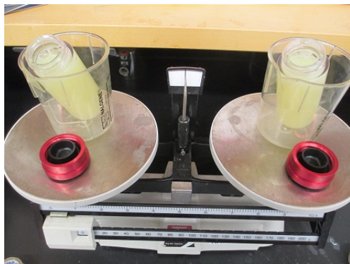
Figure 7. Cell lysates in the ultracentrifuge tubes (step E7). Two tubes need to be balanced precisely.
