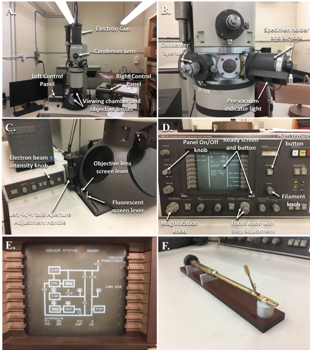
Figure 9. Phillips CM10 Transmission Electron Microscope. A and B. A general overview of the electron microscope and its parts. C. The left control panel is mainly used to control the intensity of the electron beam and for adjusting the screens for focusing images with the objective lenses or capturing images by lifting the fluorescent screen. D. The right control panel houses most of the functions needed for adjusting magnification, focusing, and the screen for monitoring the electron microscope system as a whole. E. The vacuum screen shows a schematic of the vacuum system with the various pumps, valves, and pressure gauges used to
