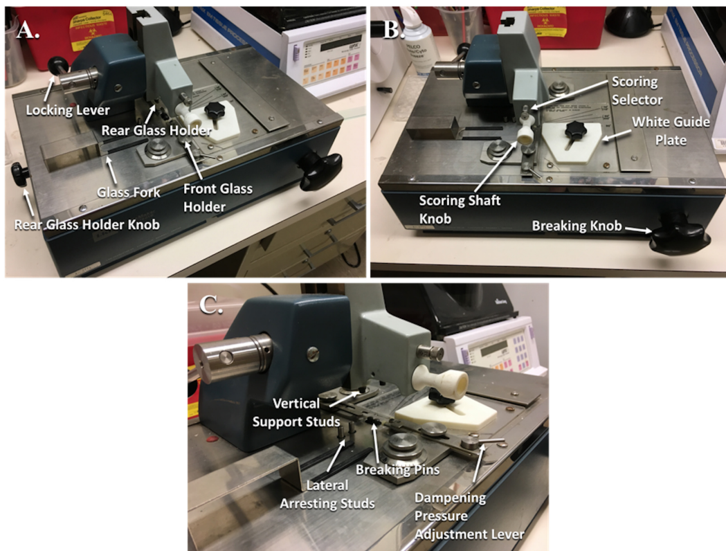
Figure 2. Glass knife maker with labeled parts. A. Angled side view with labeled parts. B. Angled frontal view with labeled parts. C. Close-up of angled side view with labeled parts.
