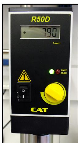
**Figure 2. Motor-driven homogenizer**
