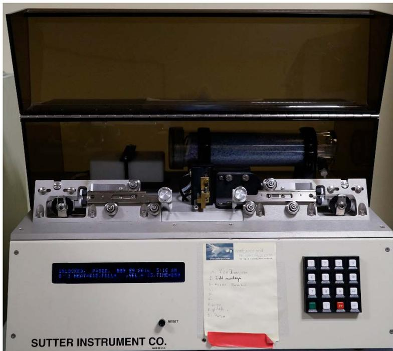
**Figure 5. Puller used for creating glass pipettes**
