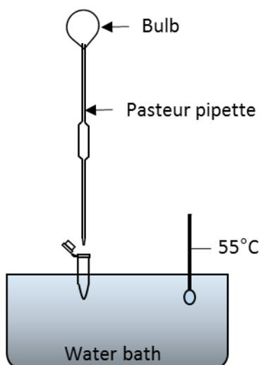
**Figure 3. Set up for drying the contents of microfuge tubes in a water bath.** After COR is extracted from bacterial culture with ethyl acetate, the ethyl acetate is evaporated by floating the tube on water bath set at 55 °C and blowing air using Pasteur pipette. Alternatively, the tubes can be left open to dry overnight.
