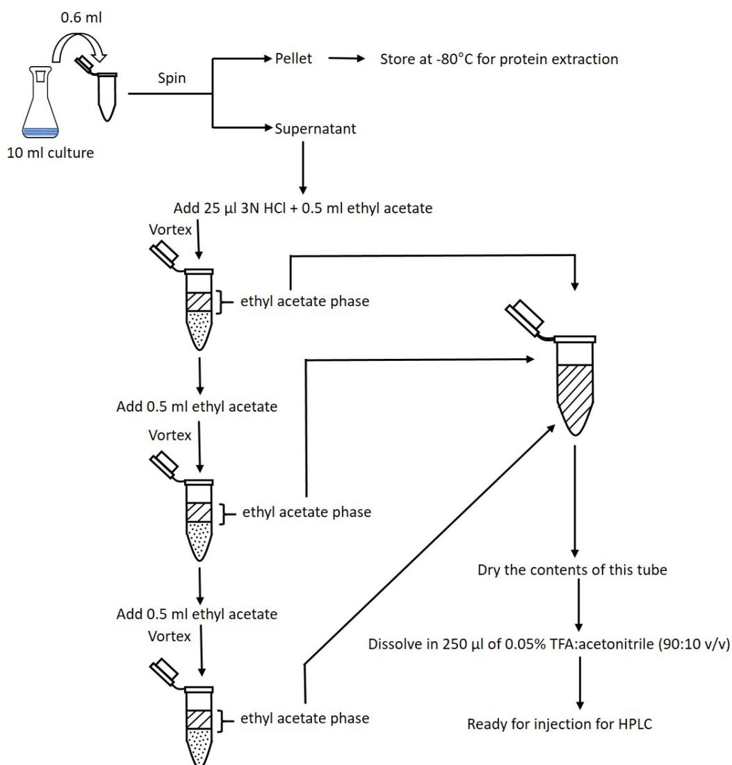
**Figure 2. Flowchart of the COR extraction.** Steps for extracting COR from bacterial culture supernatant using ethyl acetate. The three ethyl acetate phases are combined in a single tube and let dry. Dried COR is dissolved in TFA:acetonitrile and this solution is now ready for injection into HPLC.
