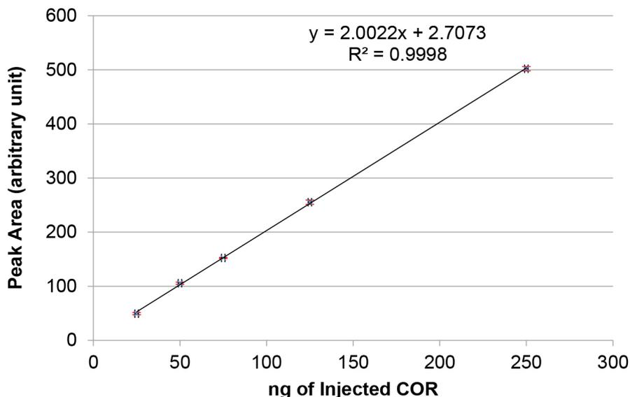
**Figure 1. Standard curve for 5-50 µg/ml of coronatine (COR).** Purified COR was injected in different concentrations and the peak area (in arbitrary units) for each injection was quantified with the chromatography data system software. Note that the red error bars for each data point are very small and do not clearly appear in the graph.
