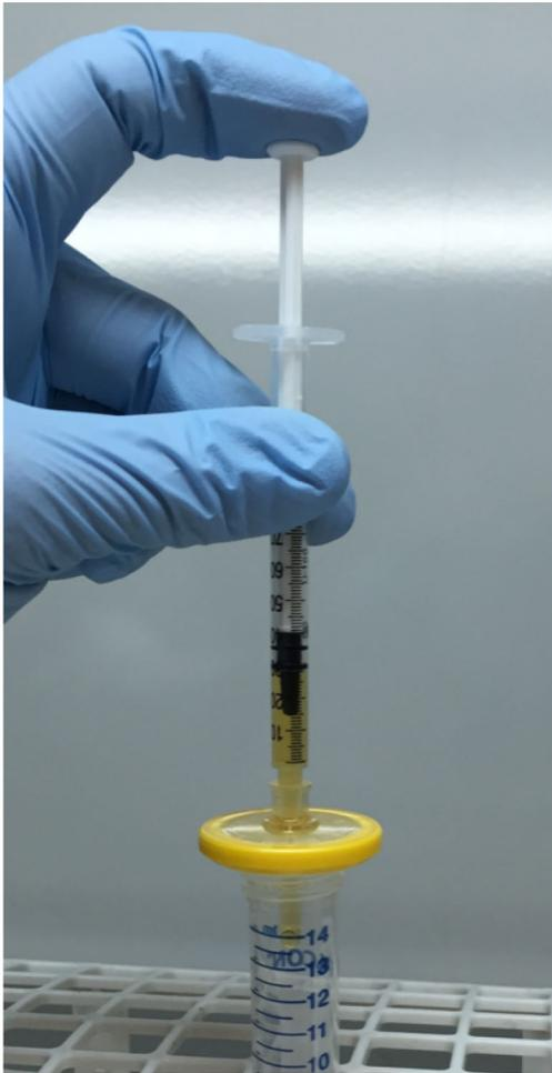
**Figure 3. Sterilization of the extract.** After centrifugation, bacteria-rich protein supernatant/extract is collected and passed through a 0.22  $\mu\text{m}$  syringe filter.
