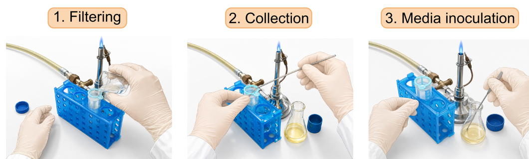
Figure 2. Recovery of alginate capsules after gelation and inoculation into fresh culture medium. The workflow comprises three sequential steps. (1) Filtering: Following capsule formation, the suspension is passed through a sterile 40 \mu m cell strainer to retain the alginate capsules and remove the CaCl 2 gelation solution. (2) Collection: The retained capsules are gently recovered from the cell strainer under sterile conditions using a sterile spoon. (3) Media inoculation: The collected capsules are transferred into a flask containing fresh, filtered YPAD medium for incubation and microcolony growth.
