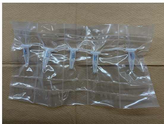
Figure 1. Lipid storage method. Partition a polyethylene roll into individual compartments using a heat sealer. Place one Eppendorf or glass tube into each compartment and vacuum-seal the roll.
