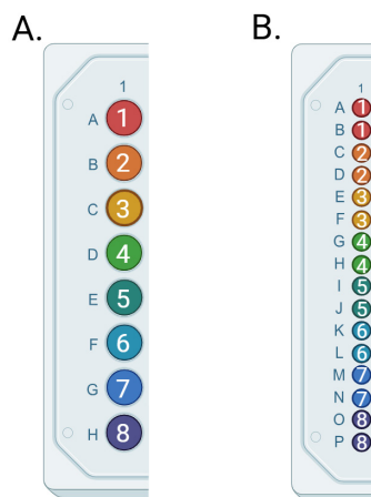
Figure 1. Example plate layouts. (A) Samples 1–8 on the 96-well dilution plate. (B) Samples 1–8 in duplicate on the 384-well PCR plate.
