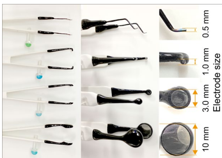
Figure 9. Types of electroporation electrodes. Electroporation electrodes should be selected based on the target region and the size of the insect. For first- or second-instar T. dichotomus larvae, 3.0 mm electroporation electrodes are used. In addition to the electrodes shown in the figure, various other types are commercially available.
