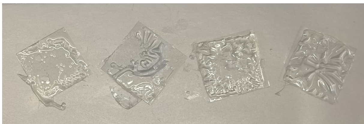
Figure 8. Structural instability of PEGDA hydrogels, which are unable to form stable structures and instantly swell after water contact
