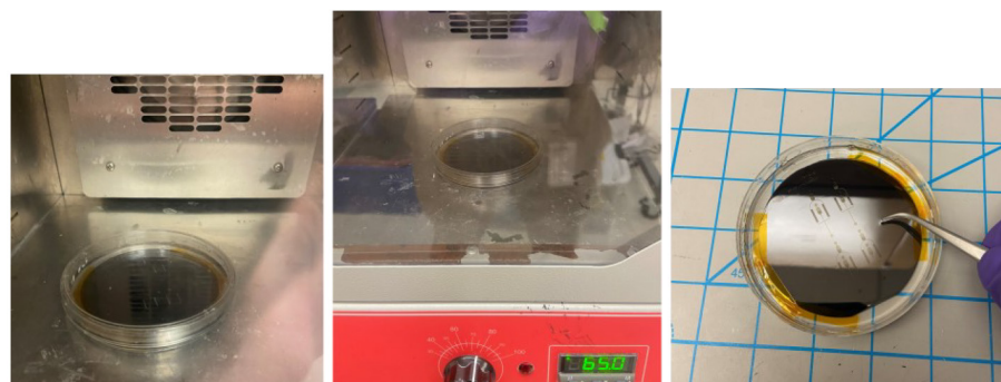
Figure 5. Stepwise procedure for oven-curing a PDMS mold
