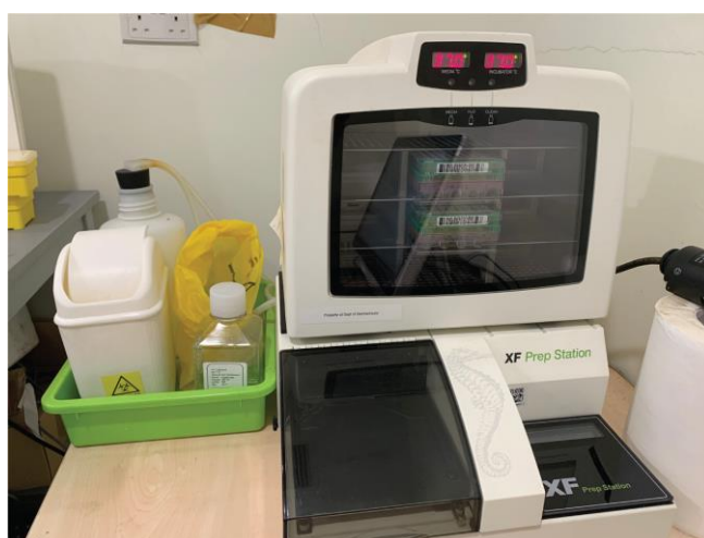
Figure 3. An example of an XF Prep Station that can be used for incubating the plates at 37 °C overnight
