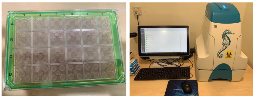
Figure 4. Seahorse XF analyzer. Left: an example of a cartridge for loading the drugs into the Seahorse XF analyzer. By default, each sample is assigned to each quadrant, where Port A can be assigned at the top left, Port B at top right, and Port C at bottom left. Right: the cartridge can then be loaded in a Seahorse XF analyzer.
