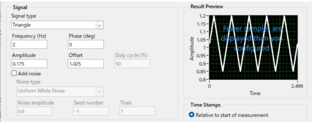
Figure 3. Setting of simulate signal express function in LabView. z-Piezo applied a 2 Hz triangle wave with an amplitude of 1.025 \pm 0.175 V using USB-DAQ.
