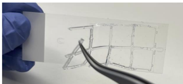
Figure 1. Silicone gasket removal. Removal of silicone gasket using fine curved forceps. Take caution to avoid scratching slide with the forceps.
