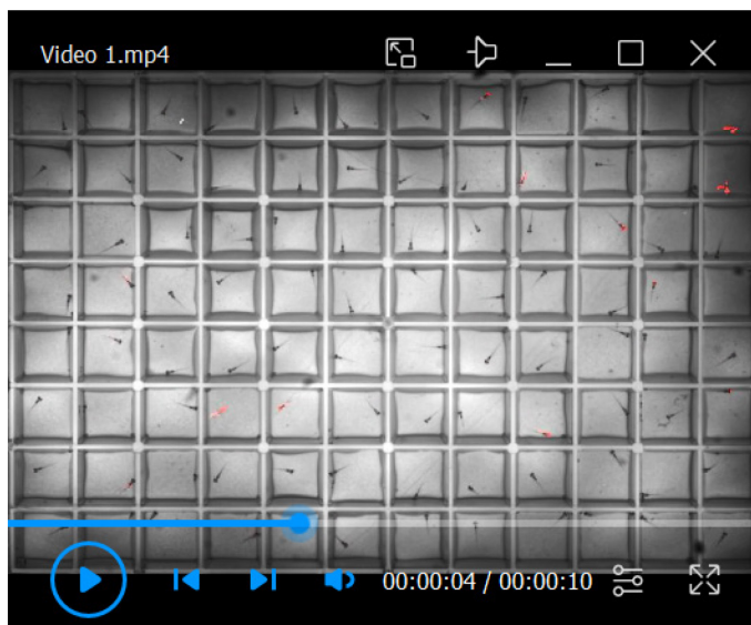
Video 1. Example of an un-sealed 96-well plate monitored using the Quantization mode with the following parameters: detection sensitivity, 25; burst (threshold for large movements), 900; freeze (threshold for no movement), 10; integration period (bin size), 60 s.
