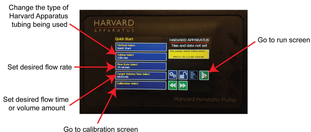
Figure 3. Run screen on Harvard Apparatus Pump.
