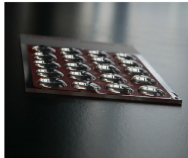
Figure 1. Preparation of a comet slide. A. A clean Trevigen® CometSlide™ HT is placed inside a plastic container. B. The comet slide is pre-coated with molten 1% agarose. This ensures that
