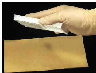
Figure 3. Flicking procedure. As described in Step F6, the plate should be vigorously flicked on a paper towel to completely remove the solution in the wells. The flicking should be repeated 5 times.
