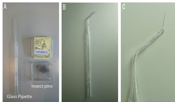
Figure 3. Preparation of insect pin. A. The required equipment. B. The finished instrument. C. A close up image of the tip.
