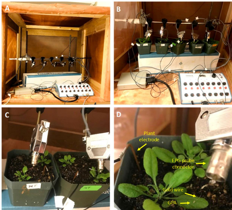
Figure 10. The EPG setup. A. A Faraday cage containing the Giga-8 setup; B. A close up of the Giga-8 setup monitoring the activity of five GPA on Arabidopsis ; C-D. A close-up view of GPA attached by the aphid electrode to the Giga-8 system.
