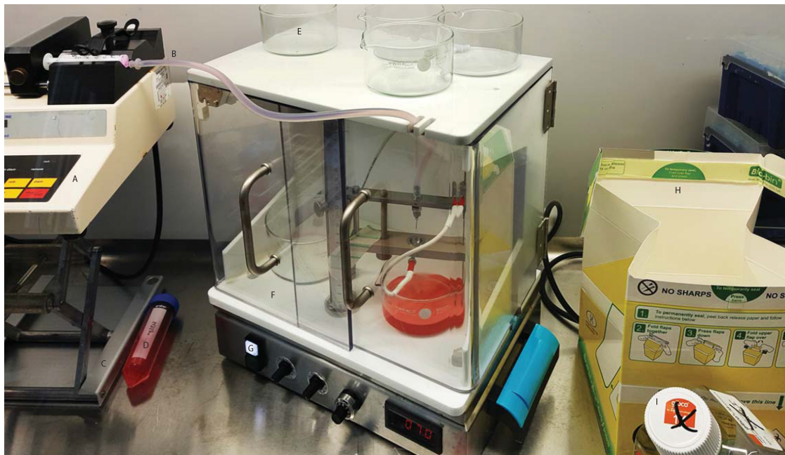
Figure 3. Bioelectrospraying microspheres. Matrix in syringe is injected to the bioelectrospraying machine and microspheres are formed. A syringe filled with matrix was set up on syringe pump (A) so that it will inject the matrix into silicon tube (B) connected to the electrostatic bead generator. The syringe driver is sitting on jack (C) for height adjustment. E. Unused crystalizing glass beakers on the roof of the bioelectrospray machine; F. Housing with doors to enclose the electrostatic bead generator; G. High-voltage switch on/off (white, on/green, off) which is left of potentiometers for optional peristaltic pump, agitator speed and voltage on electrode. Voltage indicator displaying 7.0 kV. Biobin (H) and old media bottle (I) containing surfanios (10%) for discarding biohazardous waste.
