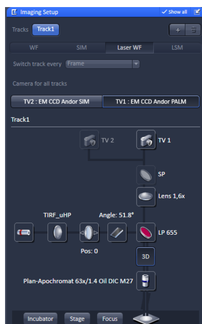
Figure 8. 'Imaging Setup' tool of ZEN 'Acquisition' for PALM. The experiment is set up for imaging with the 642 nm laser line using the ultra-high power field (uHP). The Andor iXon897 camera is selected by 'choosing the 'TV1: EM CCD Andor PALM' button.
